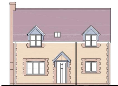
west/road elevation 1:100 Elevations - Norfolk red brick rubble flint or chalk or coursed carrstone Roof - Clay pantiles to main roof and clay plain tiles porch canopy
